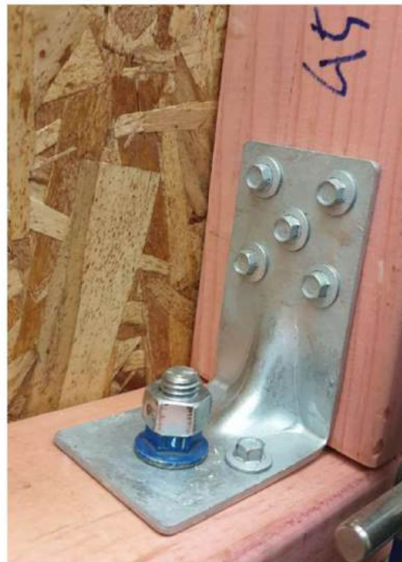
Figure 2. Bracing brackets. Note – small gap under stud is after testing on 1200 mm sample.
